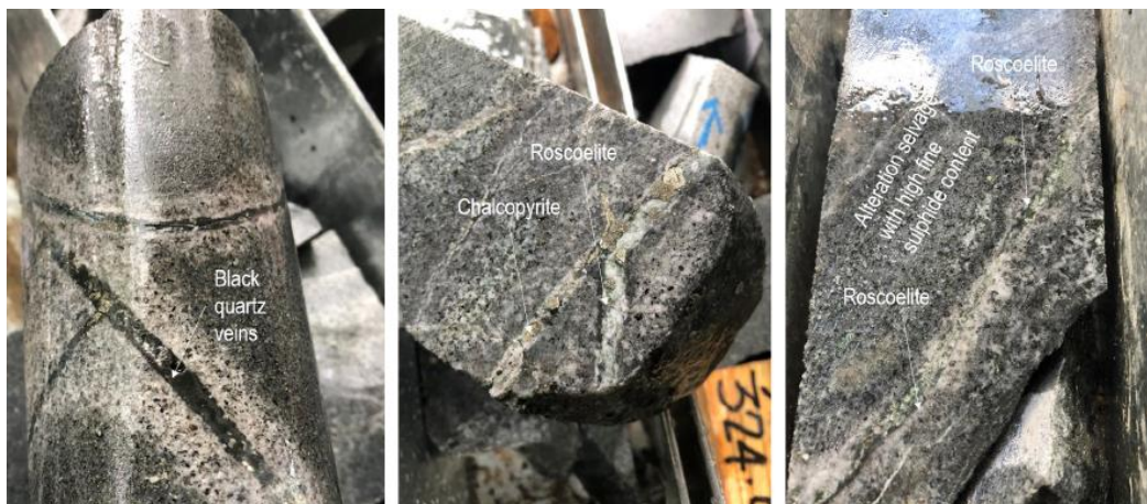
Figure 1: Examples of veinlets encountered over a 11.3m interval beginning at 318.6m in diamond drill hole TUDDH493. This intercept is situated approximately 7m from a high-grade intercept encountered in historic hole TUDDH160. Green roscoelite, an indicator mineral, is evident in some veinlets.
