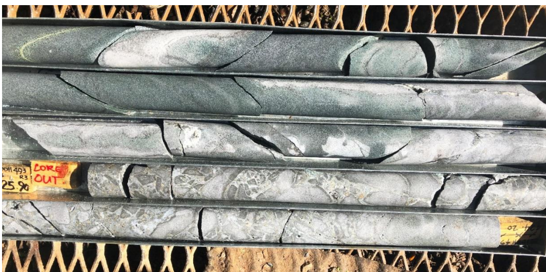
Figure 2: Hydrothermal breccia encountered between 422.5m - 426.5m in diamond drill hole TUDDH493. Monzonite fragments are intensely potassically altered. Cement is comprised of quartz-adularia-pyrite. Small pits called vugs are evident, some containing small particles of gold.
