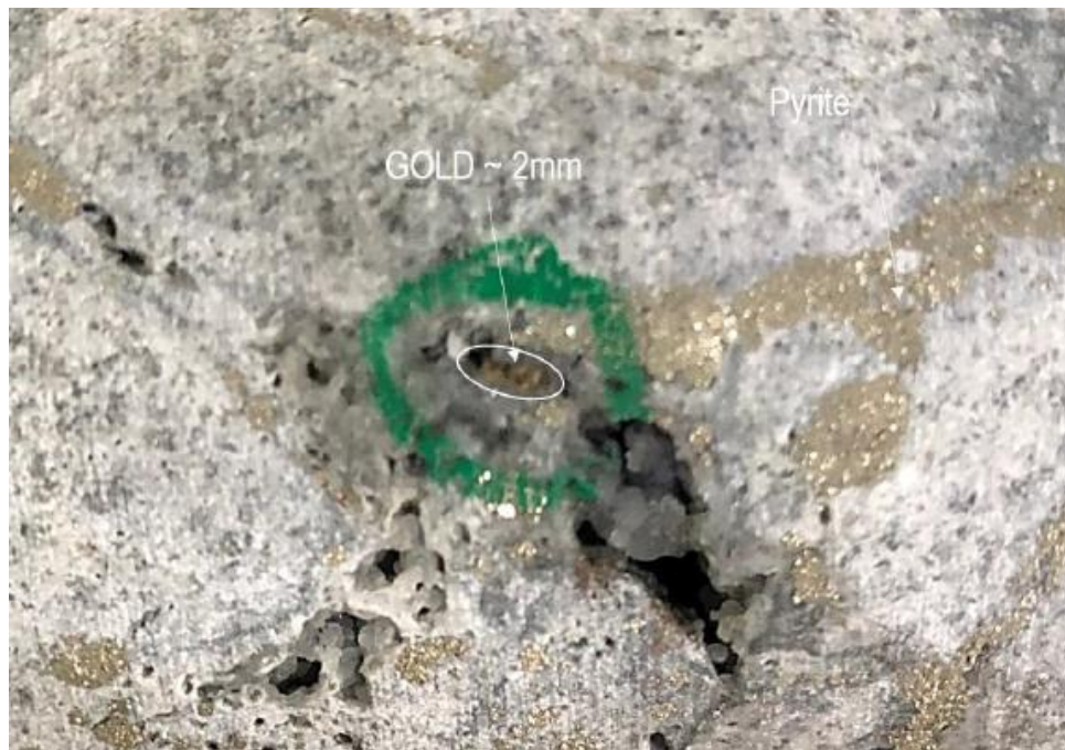
Figure 3: Two mm cluster of crystalline gold in a small vug at approximately 423m, hole TUDDH493. Such mineralization is typical of high-grade at the nearby Vatukoula Mine. Lion One believes the mineralizing system at Tuvatu is evolving with depth, perhaps becoming higher grade.
