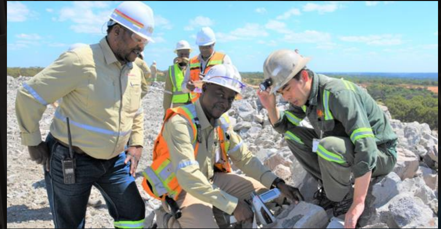
(L-R) Magloire Kashiba (Production Manager), Didier Masengo (Senior Mine Geologist) and Qiao Wei (JMMC Production Manager) examine samples of ore on the high-grade stockpile with a portable Niton analyzer (X-ray fluorescence)
