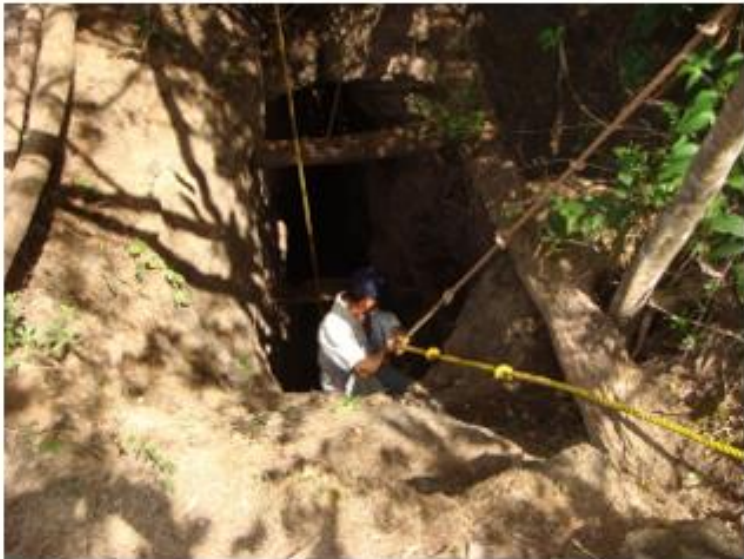
Fig. 8.20 Historic stope at San Agustin. A grab sample of the dump next to this stope carries values of 682 g/t Ag and 18.14 g/t Au (sample 19140).
