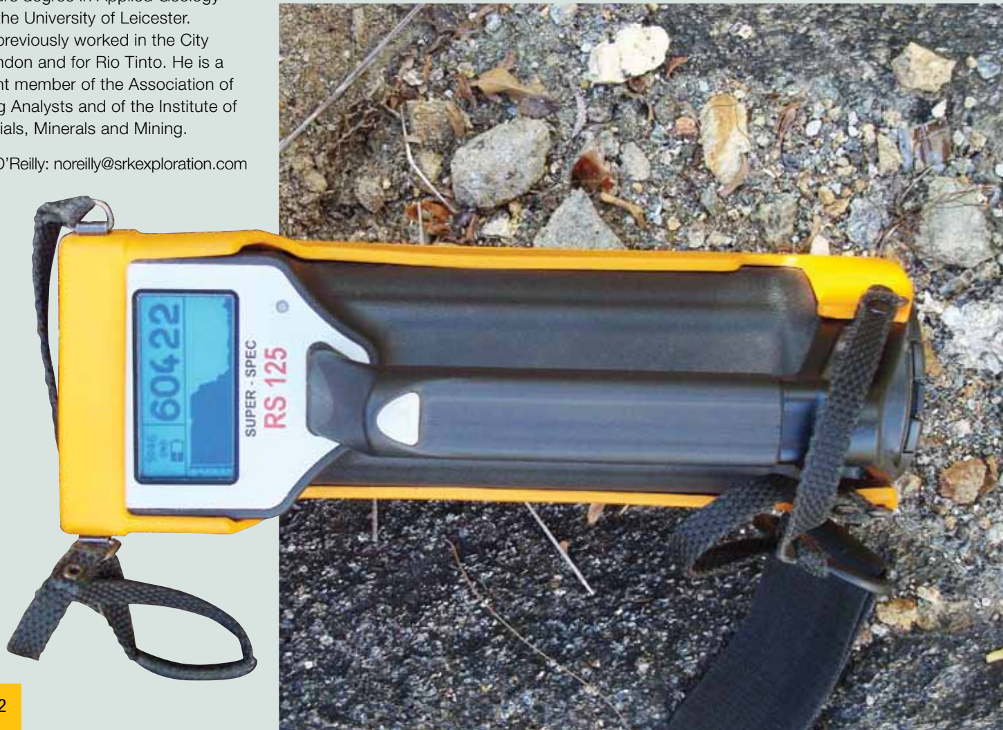
Spectrometer measuring very high natural radiation from a Uranium rich skarn in southern Africa
