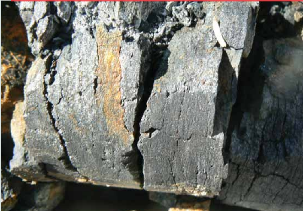
U(VI) minerals and pyrite oxidation products in Karoo shale hosted uranium ore, Botswana
