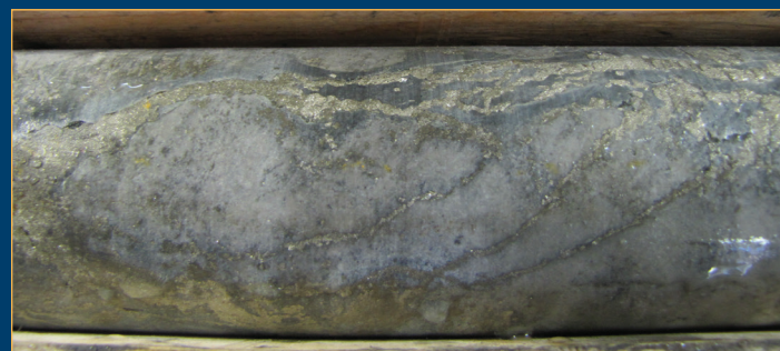
Drill core of volcaniclastic and brecciated rocks of the Blackwater deposit exhibiting mineralization.
