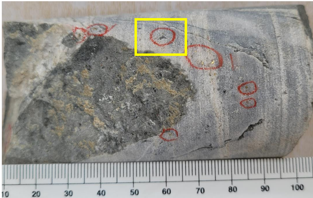
Photo 1: SDDSC061 at 691.2 m with multiple points of visible gold shown in the red circles. Yellow box shows the location of Photo 2. Scale in cm.
