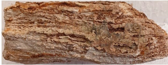
Sinter clast from hydrothermal breccia
