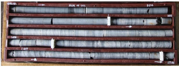
Massive grey anhydrite unite in hole TSN1-007
