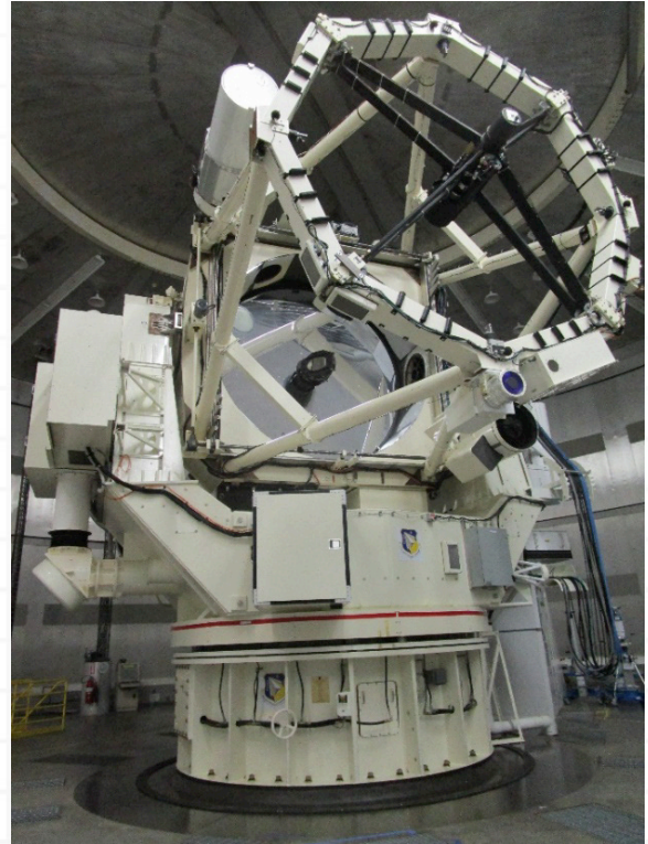
The 3.6-meter, 75-ton Advanced Electro-Optical System (AEOS) telescope shown above is the largest optical telescope in the Department of Defense. In addition the Maui Space Surveillance System facility houses several other telescopes ranging from 0.4 to 1.6-meters. Photo credit: AFRL
